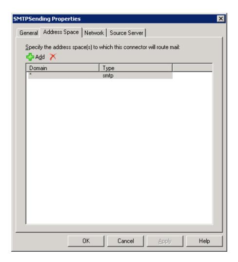
The Address Space tab shows the addresses which will be routed by the connector. It should be set to Domain \* with a type smtp.
