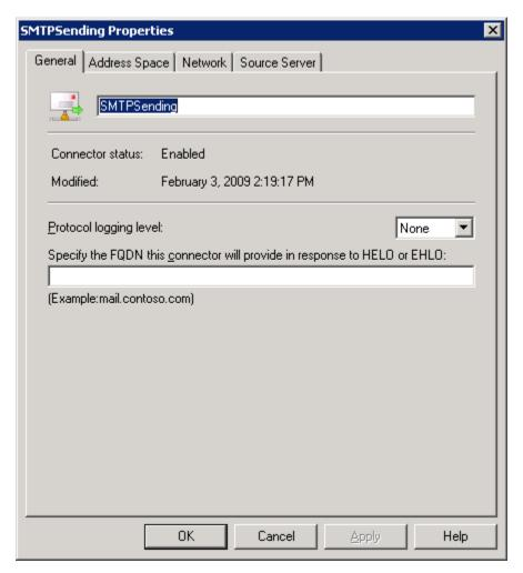
The general tab will give the name of the send connector. Note the connector's name - in the example above it is "SMTPSending".
