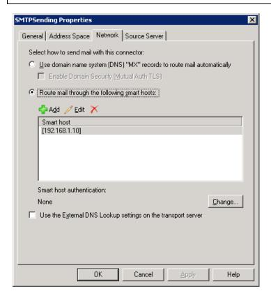
Make sure that **Route mail through the following smart hosts** is selected and that the Smart host is showing the IP address or computer name of the eXchange POP3 computer. If not, select the Smart host entry and press the Edit button.
