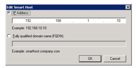
Edit the IP address or machine name to match that of the eXchange POP3 computer.
