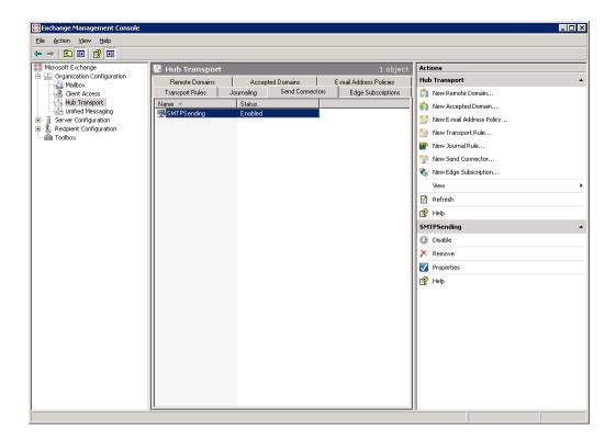
The new Send Connector is now shown. Note the connector's name - in the example above it is "SMTPSending".
