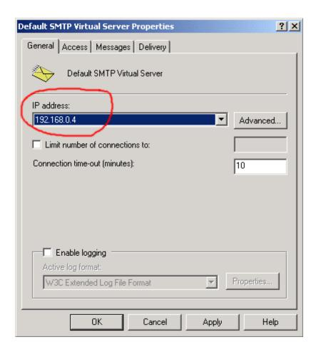
Make note of the IP address shown in the **IP Address field**. The value will either be an IP address (example: 192.168.0.4) or be 'All Unassigned'. You will need to know this value later when configuring eXchange POP3.
